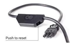
A thermo bimetallic strip, which has the advantage of being immune to high inrush currents and line transients, is heated by over current and deflects thereby releasing the latch mechanism. The contacts open even if the reset button is manually held in the closed position. This is known as trip-free mechanism. The contacts open and close with a positive snap action and the tripped state is clearly indicated by the extended projection of the reset button.
